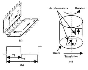
Fig. 3 Accelerometers Mounted on Drum
